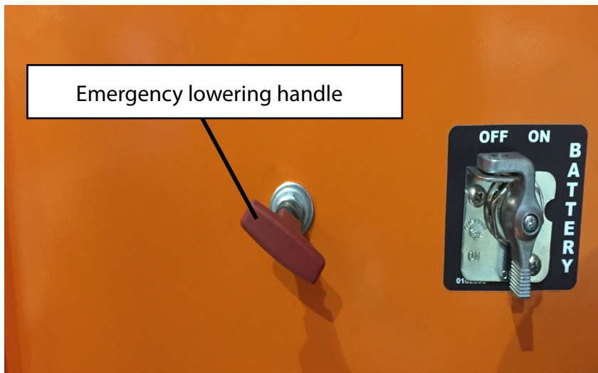
Figure 2-8: Emergency Lowering handle.
